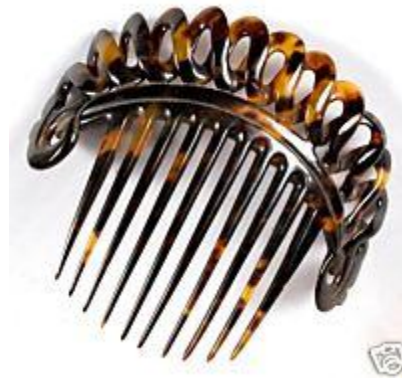
Picture 3: Hair comb of moulded tortoiseshell showing the plastic properties of the material
